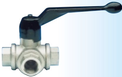
3-way full bore ball valve, L-port , with 4 P.T.F.E. gaskets, nickel-plated.
