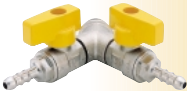
Twin-bodied ball cock L.P.G., male/2x hose connector 8 UNI 7141-72, with aluminium lever yellow plastic coated, nickel-plated.
