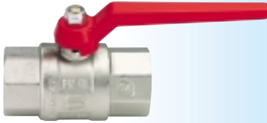
Full bore ball valve, heavy line, female/female, with face to face dimension to DIN standard 3202 Teil 4.
