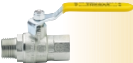
Full bore ball valve for gas with steel lever , male/female, nickel-plated.
