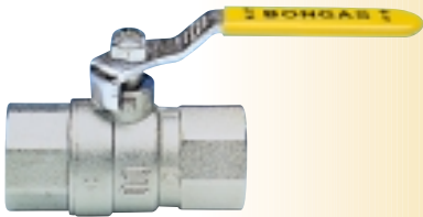
Reduced bore ball valve for gas with steel lever, female/female, nickel-plated.
