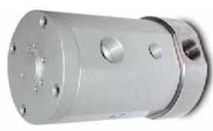
a 3 vie fil G 1" max 100 bar 100 bar max 3 ways thread G 1"
